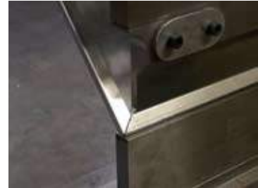
geschlossenes Blechprofil / closed plate profil
